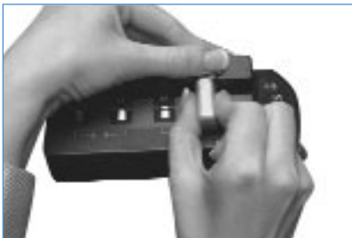
FIGURE 22: Removing the Auria™ PowerCel™ from the Charger
